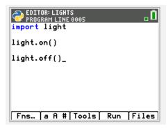
8. Add the light.off() command after the light.on() command. It is okay to skip lines in the Python Editor. They have no effect on the execution and they make the code easier to read. Run the program again. Do you see the LED blink quickly? Too fast?
