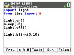
**Teacher Tip:** The **blink()** function has a tool tip when '*frequency*' is selected: 0.1–20 Hz. Hz stands for Hertz and means 'cycles per second' so a frequency of 3 means that the LED will blink 3 times in one second. The '*time*' parameter (0.1–100 s) tells the TI-Innovator Hub for how many seconds to blink. So, this is a simple multiplication example: light.blink(3,5) will make the LED blink 3\*5=15 times in 5 seconds.
