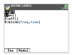
**Teacher Tip: light.on()** is a much more complex statement than it looks. **light** is an instance of a class created within the **ti\_hub** module and **.On()** is a method of the class that turns the light on. On the surface, it is an easy command to use, but underneath there is a lot of work going on. This is the power of Python at work: it makes physical programming accessible to even complete beginners.
